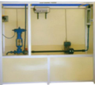
FLOW CONTROL LOOP TRAINER
